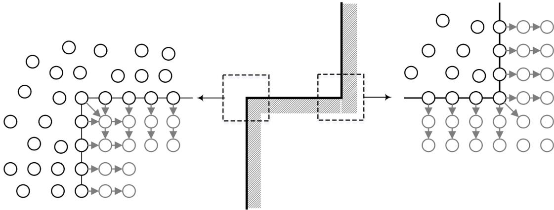
Figure 2: Calculating the wall markers pressure as suggested in [4]. The pressure of a markers located on the wall is calculated similar to the fluid markers and then projected to the interior wall markers. For an external corners, a wall marker may be influenced from several surfaces; therefore, the final pressure is an average of partial contributions.
