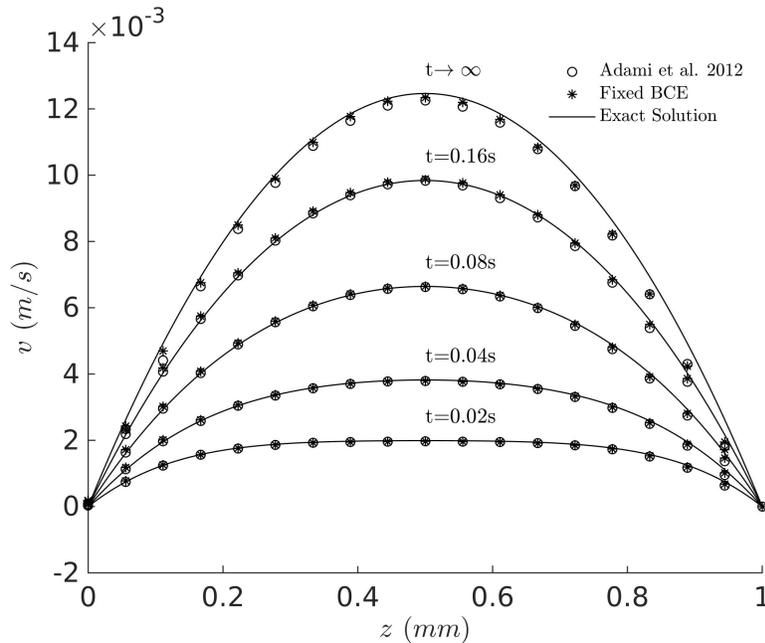
Figure 3: Transient Poiseuille flow solution obtained from *Approach 1* (\*), *Approach 2* (o), and exact solution (solid line). No-slip condition is satisfied by both simulation approaches.
