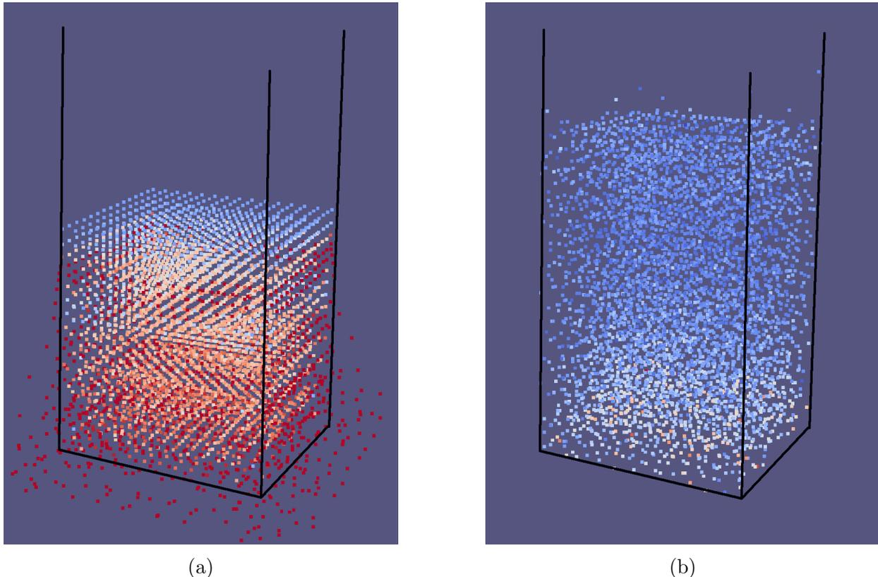
Figure 4: Test of boundary condition for no-penetration under gravity. While all simulation parameters were maintained similar, two different BCE approaches were used: (a) *Approach 1* (fixed BCE approach); (b) *Approach 2* [1]. The colors represent the markers pressure, with red and blue being the maximum and minimum pressures, respectively. The result show a clear advantage when *Approach 2* is leveraged.
