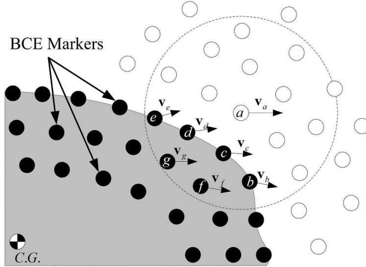
Figure 1: BCE and fluid markers, key for the coupling between fluid and solid, are represented by black and white circles, respectively. A section of the rigid body is shown herein as the gray area. The BCE markers positioned in the interior of the body (markers  $g$  and  $f$  in the figure) are placed at a depth less than or equal to the size of the compact support associated with the kernel function  $W$ .
