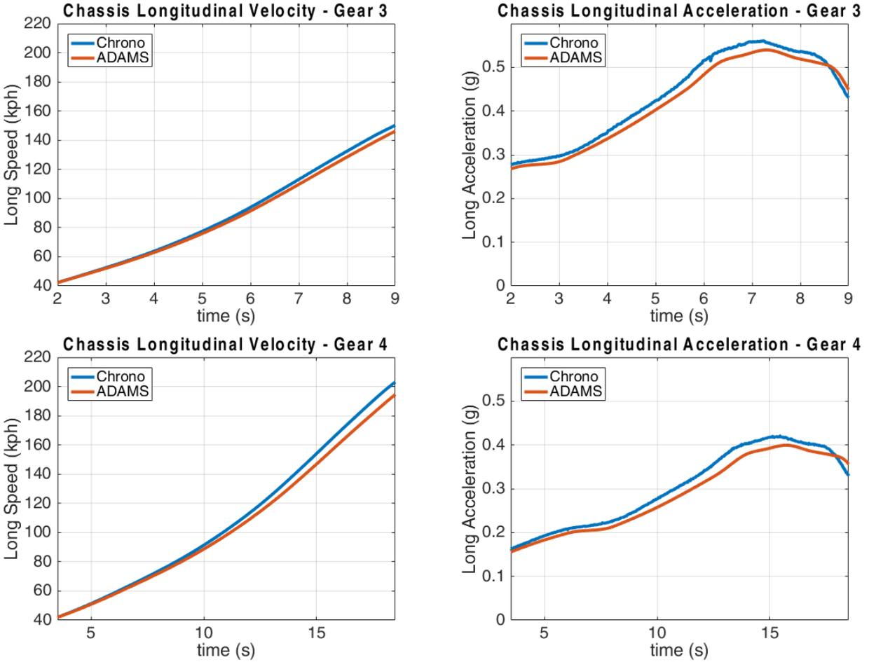
Figure 1: Straight-line acceleration test comparison between Chrono::Vehicle and MSC ADAMS/car in both 3rd and 4th gears
