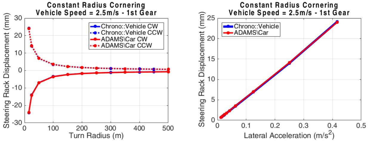
Figure 2: Constant radius cornering test comparison between Chrono::Vehicle and MSC ADAMS/car at 2.5 m/s in 1st gear
