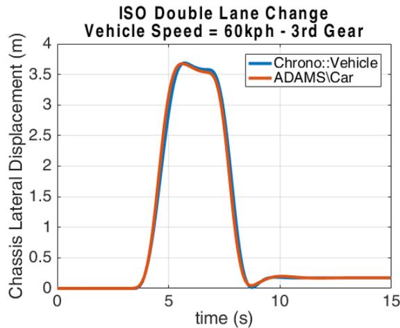
Figure 3: ISO double lane change test comparison between Chrono::Vehicle and MSC ADAMS/car at 60 kph in 3rd gear
