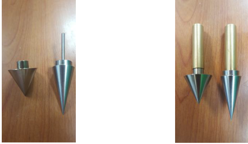
(a) Cones with 60° and 30° in the apex angle. (b) Cones with LVDT connectors attached.
