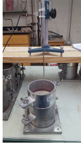
(b) One of the containers used in the experiment filled out with the granular material. The measuring apparatus is placed above it. Picture was taken right before one of the tests was conducted on.
