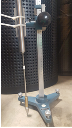
(a) Cone (with 30^\circ in the apex angle) attached to the LVDT connector. The rod putting a kinematic constraint on the cone's motion and rod's track can also be seen in this picture.
